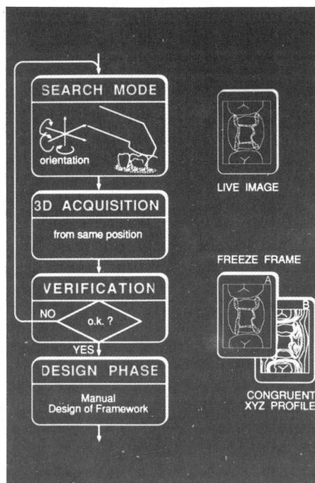
Fig. 4. Flow diagram showing the specific Cerrec »optical impression« method.
