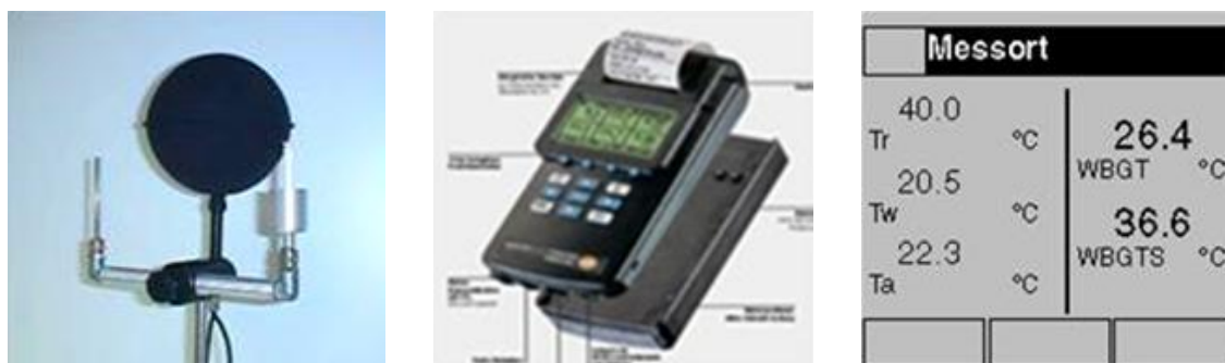
a) Sensor WBGT, b) Measuring device, c) Display readings from the measuring device
