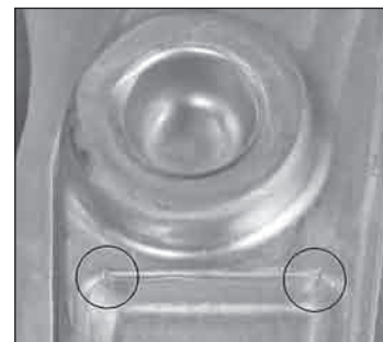
Figure 7 Overlapping present in the product after initial operation
