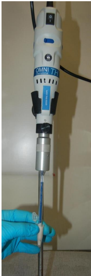
Figure 3.7 Homogenisation of tissue sample in buffer using an electronic homogeniser
