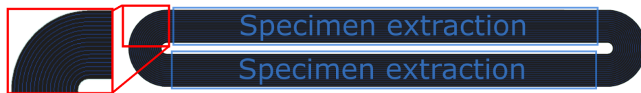
Figure 2: Print schematic of unidirectional tensile and flexural specimens showing fibre path
