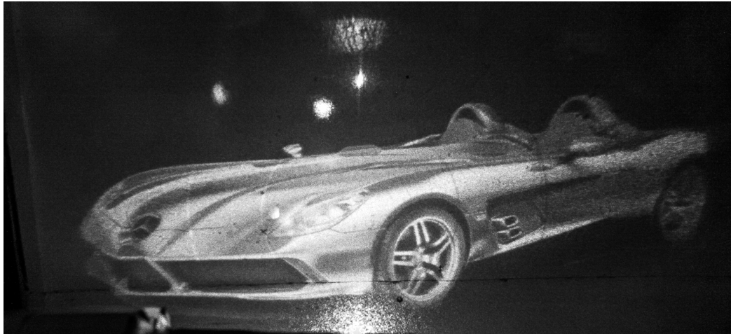
(a) Replay field with a tilt mismatch visible
