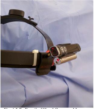
*Fig 4.5 B: Detail of Head Cam and Laser direction indicator*
