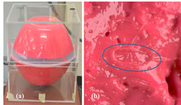
Fig. 6. (a) Entire phantom setup. (b) Indentation of capsule in phantom.
