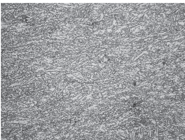
Figure 4 Microstructure of the steel no. 227 – the end of rolling at temperature 780 °C, cooling rate is 30 °C/s; mag. x1000
