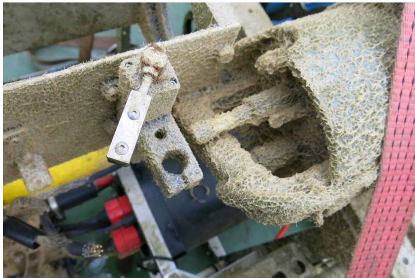
Figure 22 - The brush of the zebra tech wiper. The battery pack had been lost
