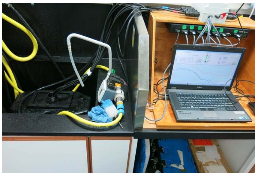
The NOC underway CO 2 system as set up near the TSG system on the main deck
