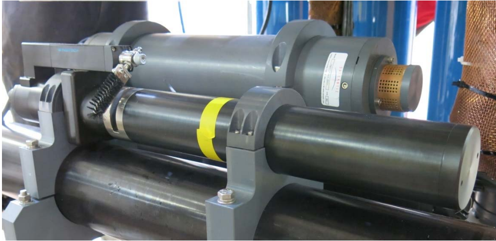
Figure 27: Satlantic SUNA S/N 745 nitrate sensor with integrated wiper ready to be deployed on a sensor frame
