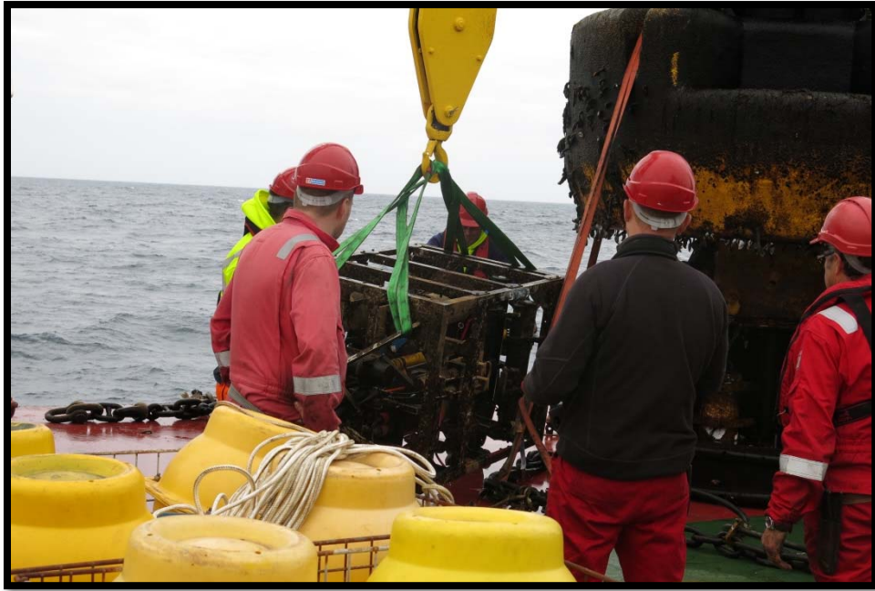
Figure 19 - Recovered system showing biofouling at the buoy and the frame.
