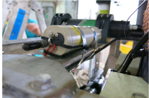
Figure 4 - Top of the frame showing the logger white housing for the load cell and the VR2W (horizontal tube) Figure 5 - CT sensor
