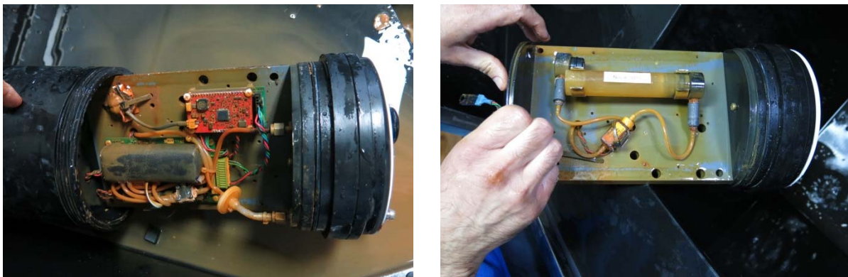
Figure 24 - Flooded sensor logger side (left) and chemical side (right)
