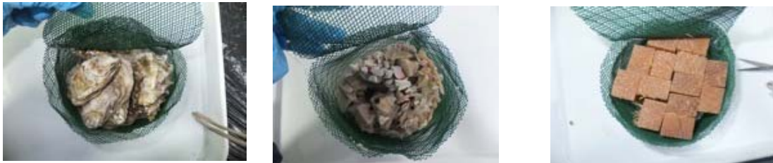
Figure 55. Experimental substrates (from left to right: shells, bones, wood) recovered from LO 3 CAted settlement frames deployed at 2997 m (top) and 4777 m (bottom) in PAP#3 mooring.
