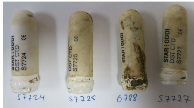
Figure 35: Recovered Star ODDI DST CTD sensors (S/N 7724, 7725, 6788 and 7727) deployed below the buoy from 28.04.2014 to 17.04.2017. Sensor 7725 did not collect any data due to a battery fail.
