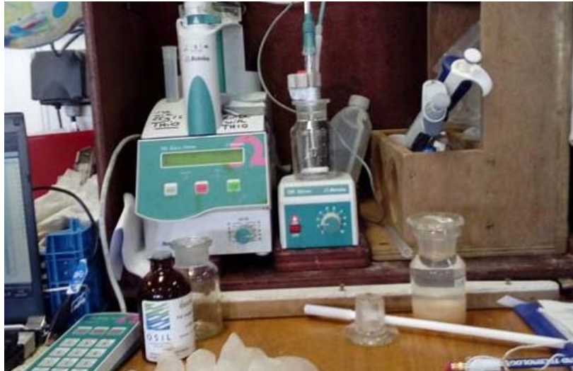
Old 'FerryBox' dissolved O 2 amperometric end point equipment set up for O 2 analysis on DY077
