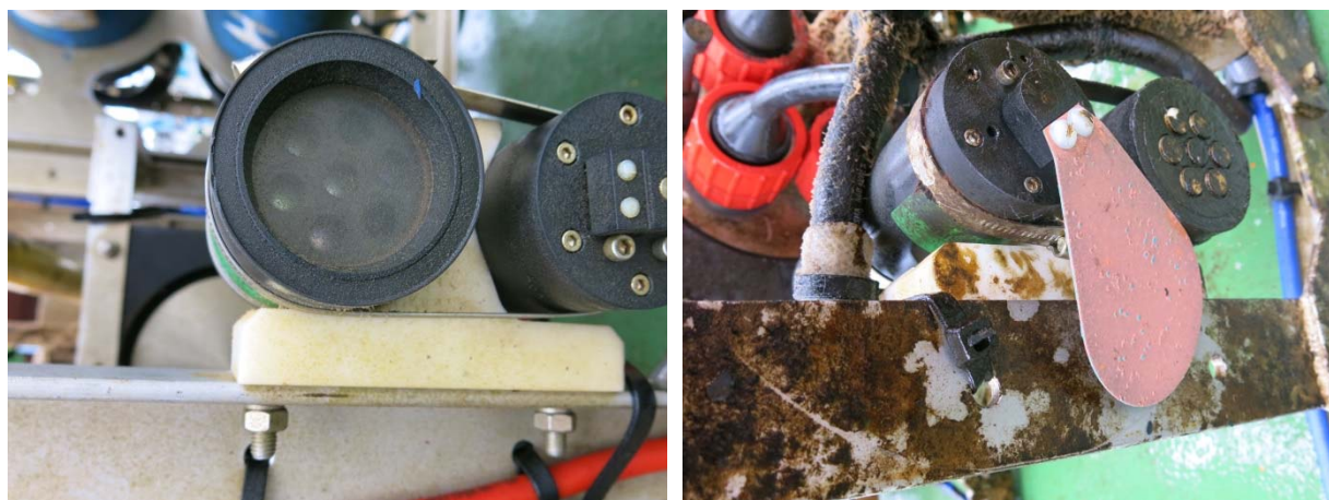
Figure 25 - OCR sensors in the frame after recovery
