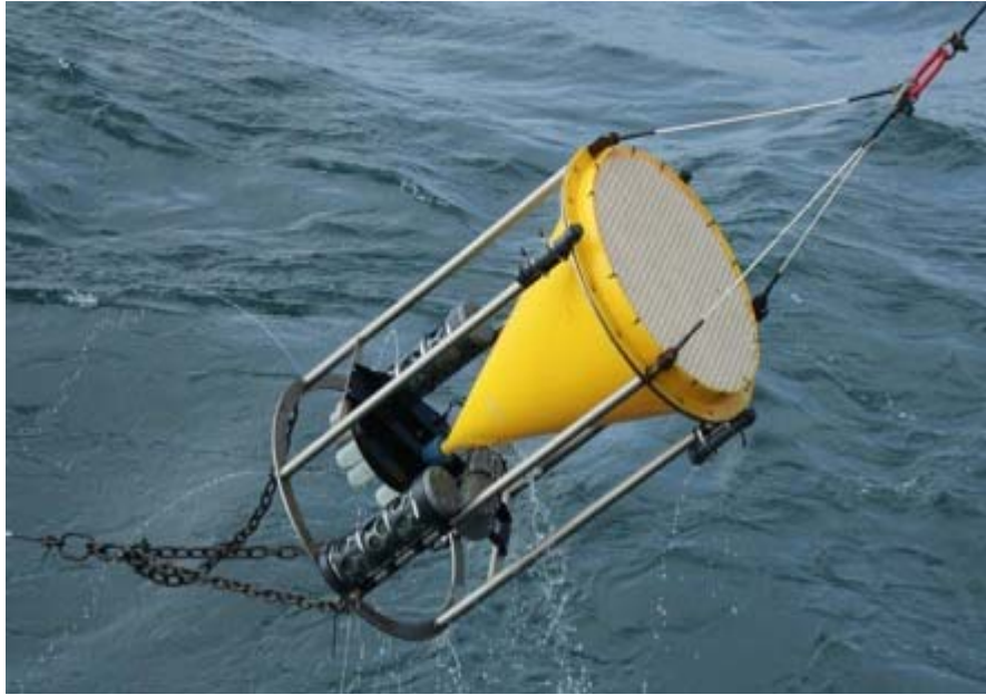
Figure 52. LO 3 CAted settlement frames and larval traps clamped to Sediment trap 2997m of PAP#3 mooring.
