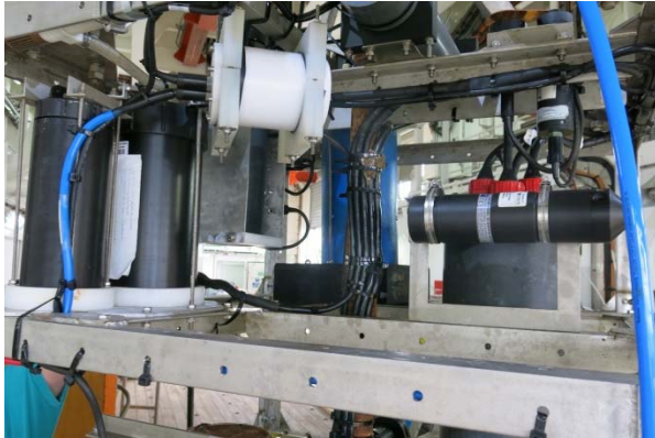
Figure 4 - Top of the frame showing the logger white housing for the load cell and the VR2W (horizontal tube) Figure 5 - CT sensor
