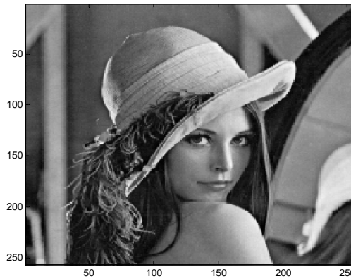
Figure 133 Reconstructed CRS encoded compressed image data with 4 errors on each packet.
