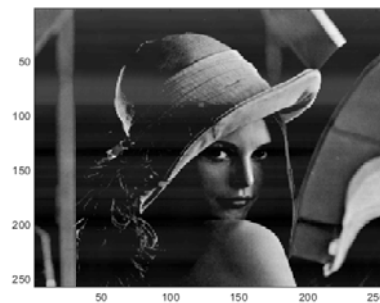
All CWT wavelet coefficients. (PSNR = 19.4513 dB)
