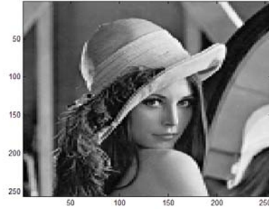
DWT \frac{1}{2} coefficients only. (PSNR = 28.9856 dB)
