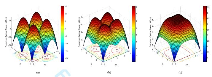
Fig. 2: Optical Power Distribution for four transmitting LEDs with (a)  $\varphi_{1/2} = 10^{\circ}$ , (b)  $\varphi_{1/2} = 25^{\circ}$  and (c)  $\varphi_{1/2} = 45^{\circ}$ .
