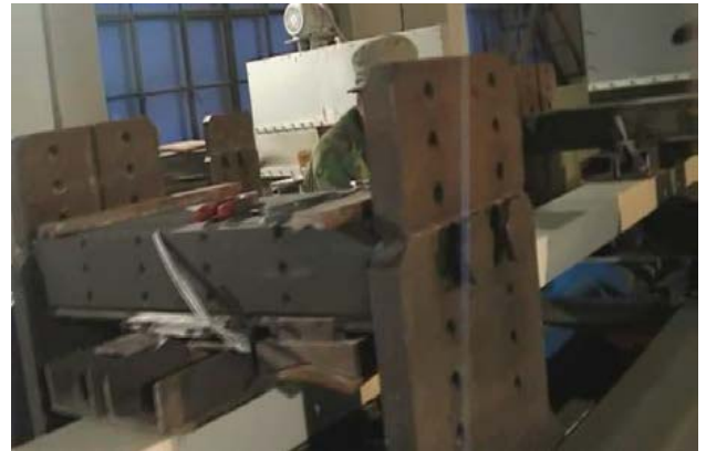
Figure 10. FRP deck pultrusion-Pull out
