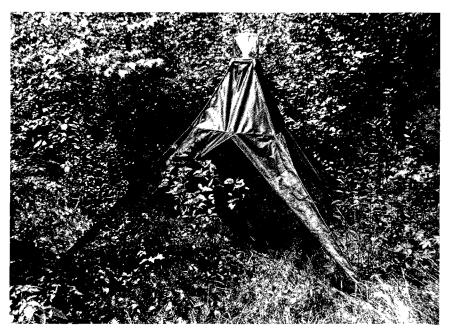
Fig. 1. Malaise trap used in this study: height to top of globe, 1.7 m; base length, center pole to corner stake, 1.2 m; base distance between stakes, 2 m; height of side openings, 1 m; color, gray-green. (Manufactured by Cornell Equipment Co., Inc., 1115 N. Rolling Rd., Baltimore, Md. 21228.)
