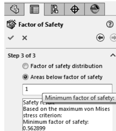
Figure 30 – Redefinition of Factor of Safety and values to be displayed on the new plot.
