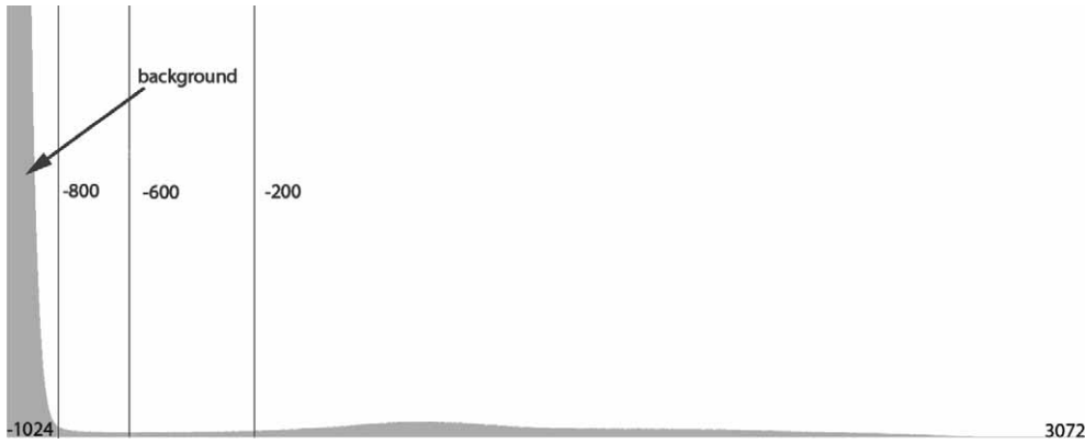
Fig. 1. Histogram from volumetric data of skull (axis x – intensity values, axis y – frequency).
