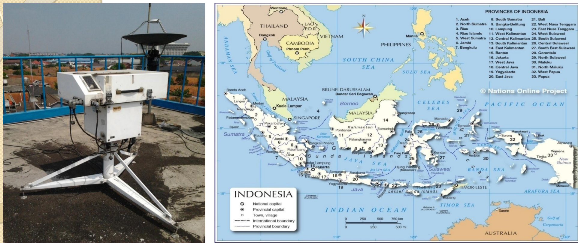
Fig. 1. Brewer spectrophotometer (left) used for the measurement of total ozone, \text{NO}_2 and \text{SO}_2 columns over Bandung, Indonesia (right) (Source: Nations online project, 2012). It was placed on the top roof of the fourth floor of LAPAN office
