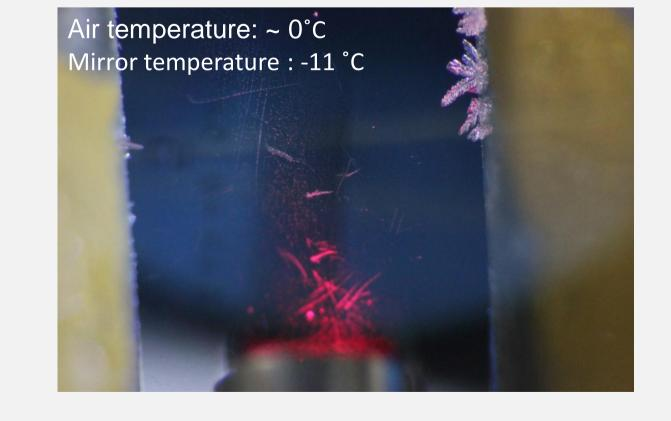
In this case, the frost at the edge of the mirror grow larger. we think that this ice is unsuitable for the good PID control, Ice should be uniform on the mirror.
