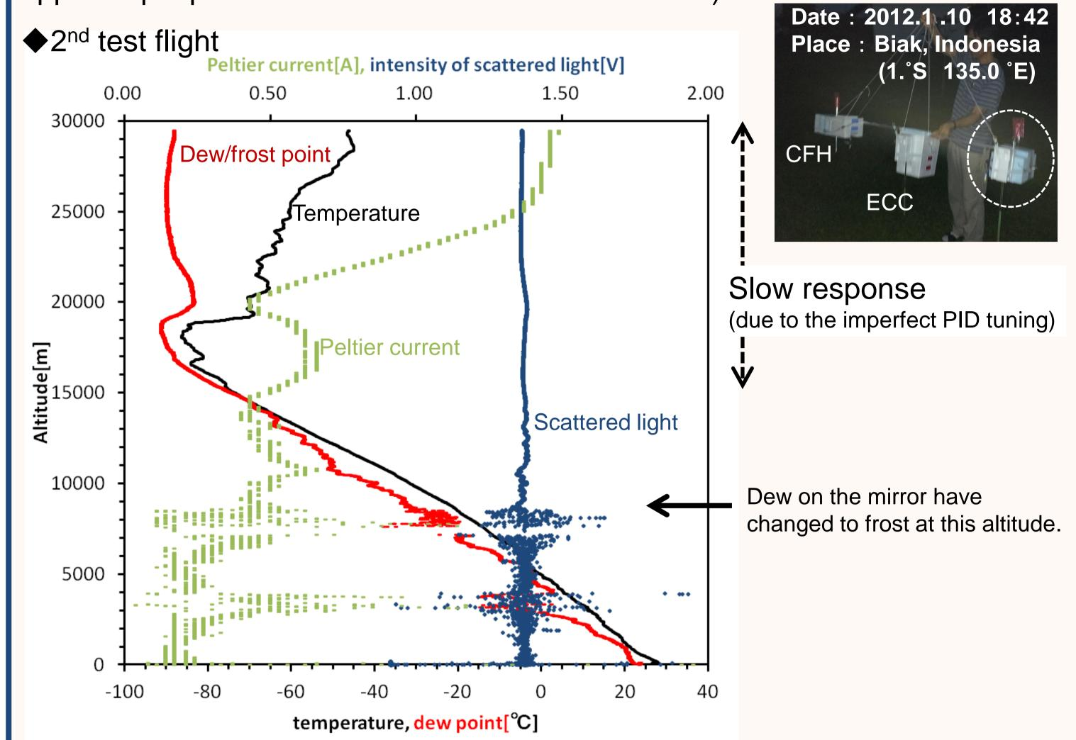
⇒ The PID tuning was changed to get a faster response in the upper troposphere and lower stratosphere in the 3<sup>rd</sup> test flight.
