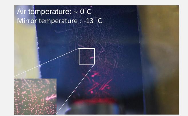
The diameter of dew is about 5 ~10 µm during operation
