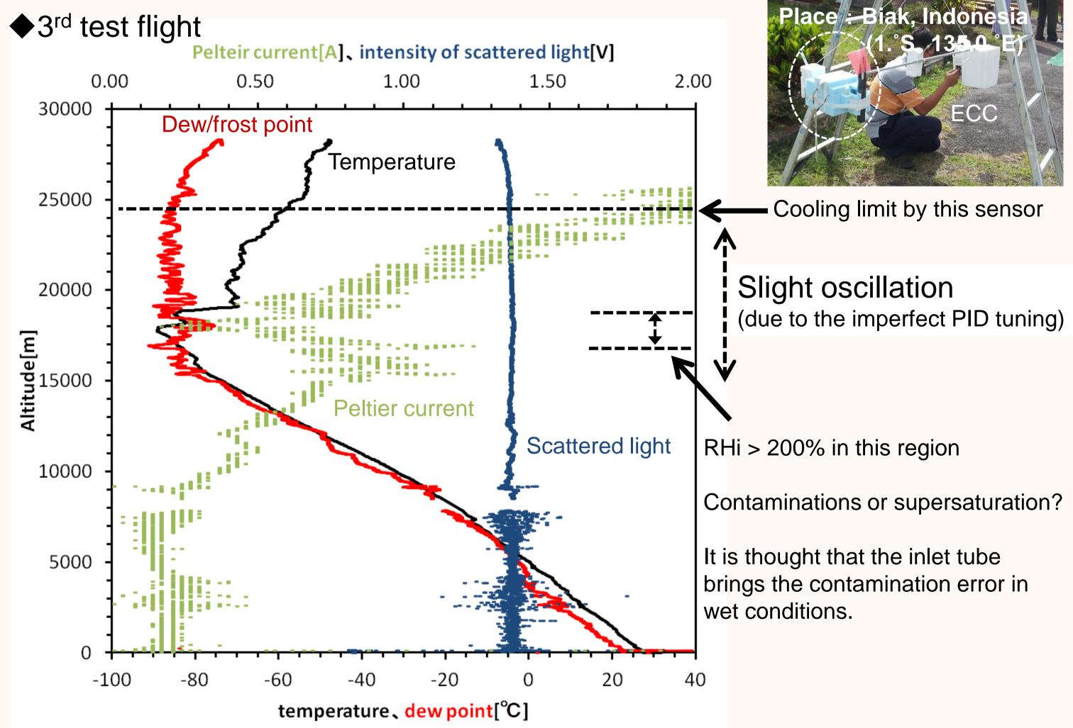
◆This result shows that our hygrometer can measure the stratospheric water vapor without cryogen at ~25 km, if we succeed in the PID tuning.
