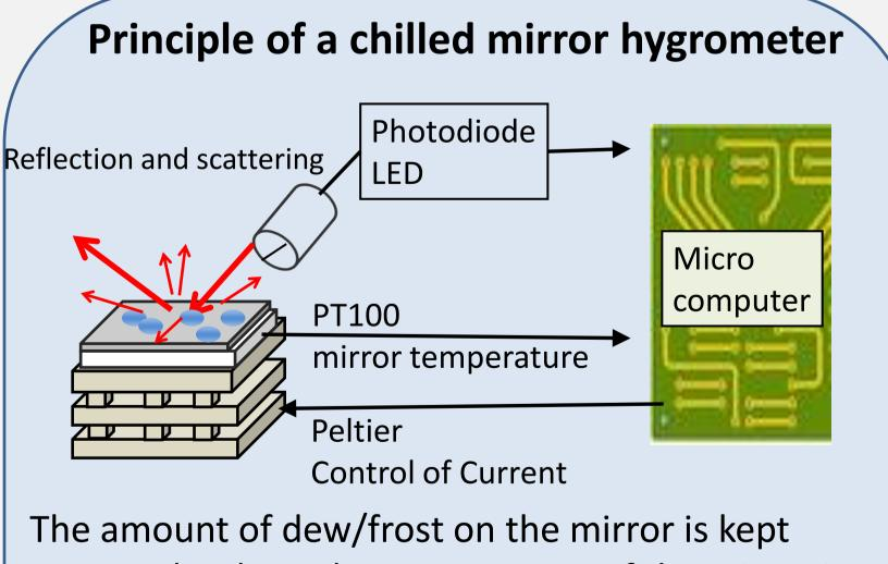
constantly. Then, the temperature of the mirror is equal to the dew point. PID controller is used to keep the dew constantly. The Peltier current is defined by a following equation.
