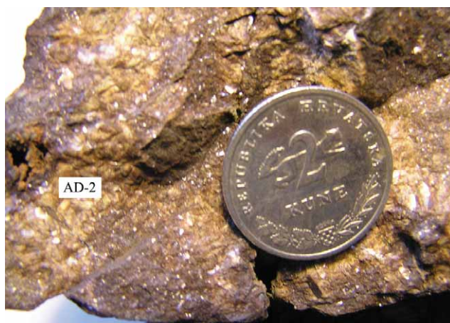
Figure 19: Yellow coarse grained siderite (sample AD-2) irregularly embedded in a matrix of reddish fine grained siderite from the Adamuša opencast mine.
