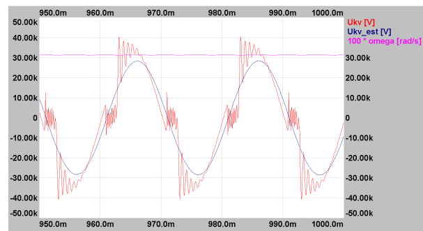
Fig. 11. Output waveforms from the modified EPLL algorithm for the estimation of the phase-angle, amplitude and frequency of the line voltage, in case of very polluted grid environment
