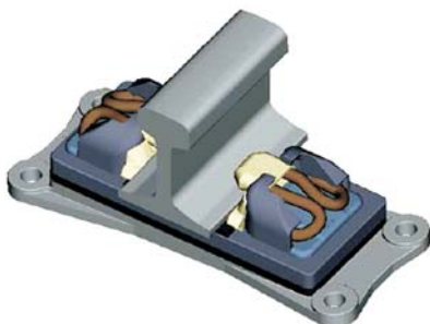
Figure 4 Resilient pre-loaded fastening system
