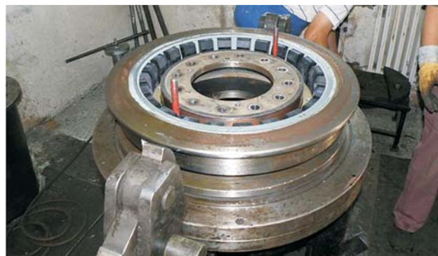
Figure 22 Resilient wheels (rubber pads installation)
