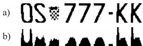
Figure 3 Vertical projection (b) of a binary license plate image (a)
