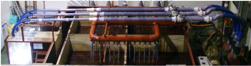
(b) Sump model test apparatus
