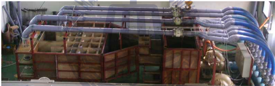
(b) Sump model test apparatus
