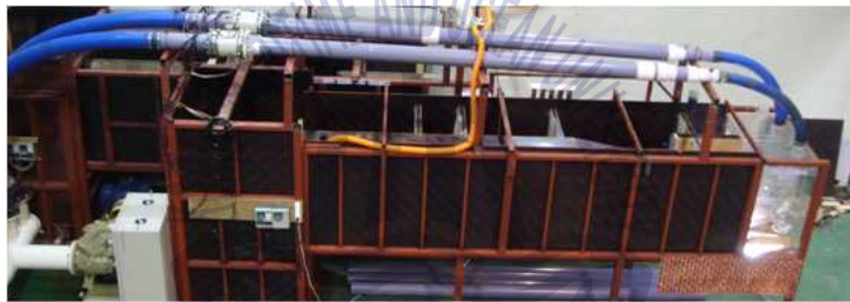
(b) Sump model test apparatus
