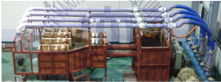
(b) Sump model test apparatus
