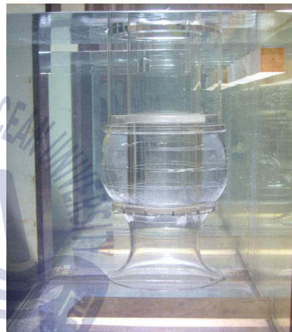
(b) Trapezoid type AVD for submerged vortex & square bar
