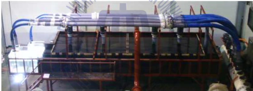
(b) Sump model test apparatus
