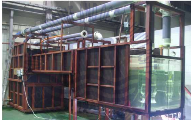
(b) Sump model test apparatus
