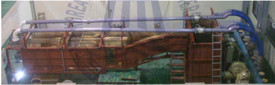
(b) Sump model test apparatus
