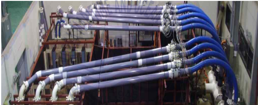
(b) Sump model test apparatus
