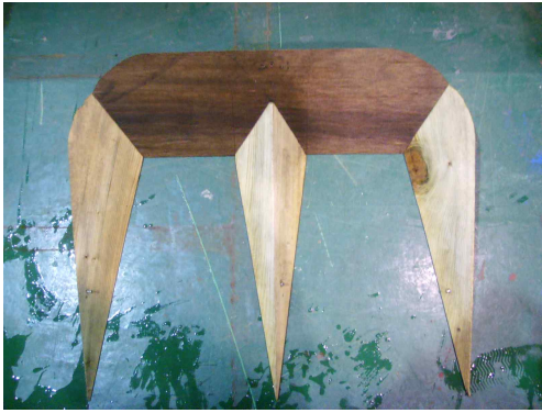
(a) HI-recommended combined type AVD for submerged vortex
