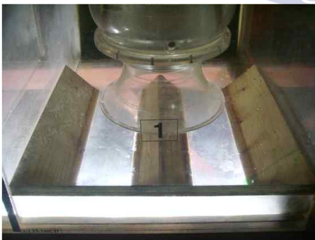
(c) KMU Lee recommended combined type AVD for submerged vortex
