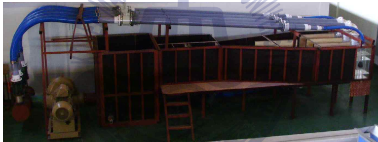
(b) Sump model test apparatus
