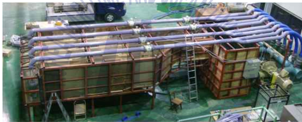
(b) Sump model test apparatus
