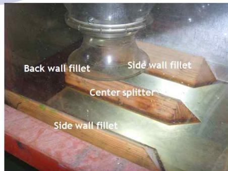
(c) KMU Lee recommended combined type AVD for submerged vortex
