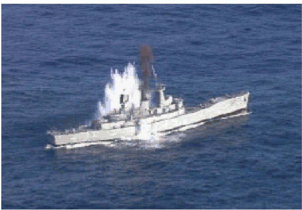
Figure 5.11 Real ship experiment of underwater explosion : the 1st gas bubble breaking
