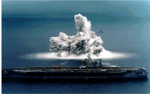
Figure 5.5 Surface phenomena of UNDEX [31]
