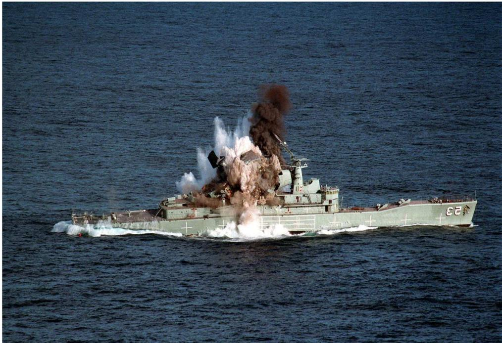
Figure 5.12 Real ship experiment of underwater explosion
