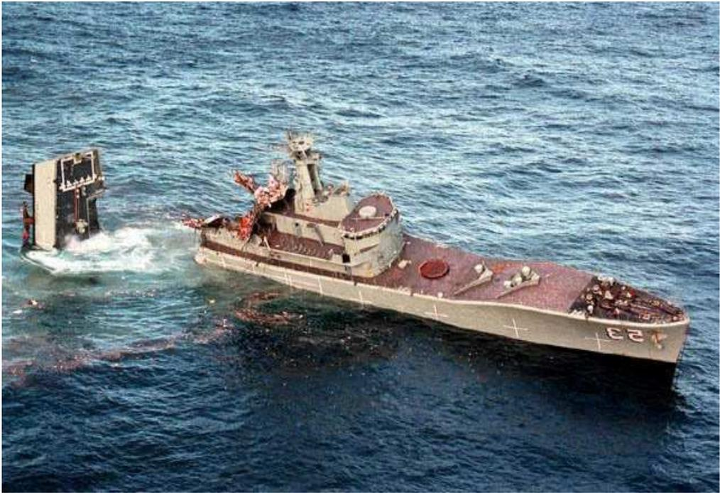
Figure 5.14 Real ship experiment of underwater explosion
