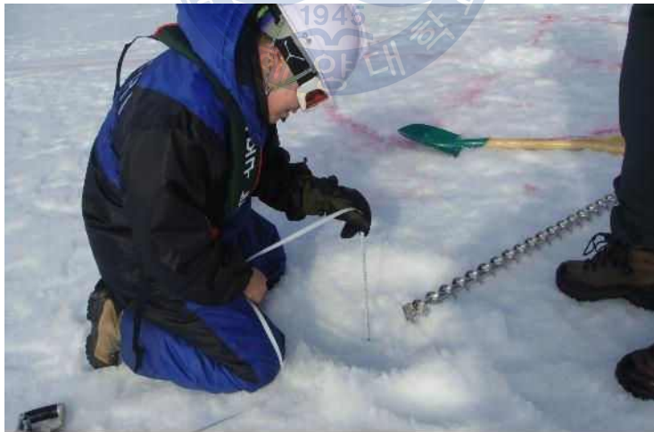
Fig. 2-6 Thickness measurement using ice gauge
