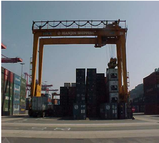
Fig. 2.5 Cargo working view of transfer crane
