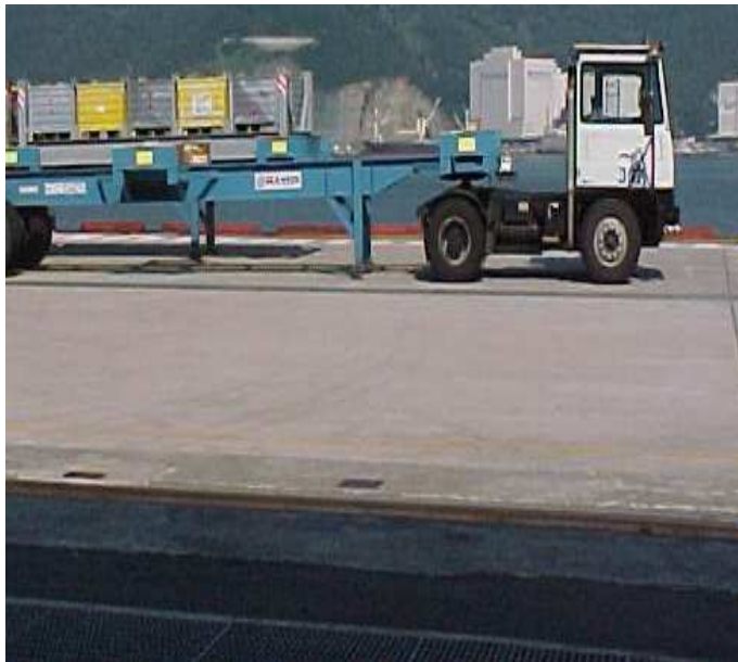
Fig. 2.7 A view of yard tractor and chassis
