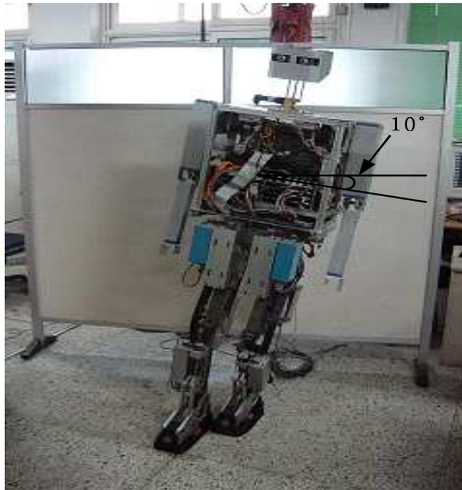
Fig. 5.26 The leaned appearance by 10 degrees while BWR is walking
