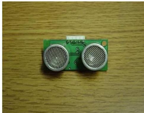
Fig. 4.4 Ultrasonic sensor system
