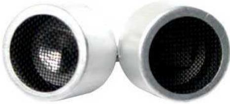
Fig. 4.3 Ultrasonic Sensor
