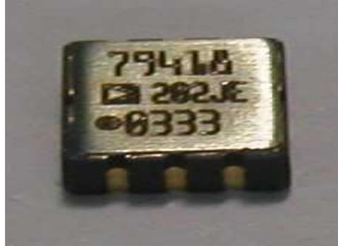
Fig 4.8 Appearance of the gyro sensor
