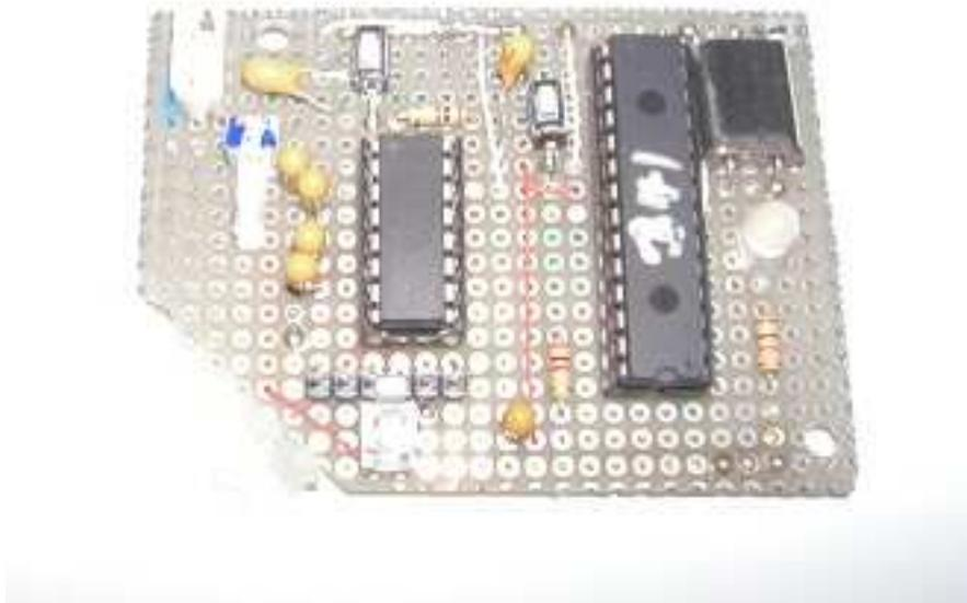
Fig. 4.20 Actuator board of the vision system
