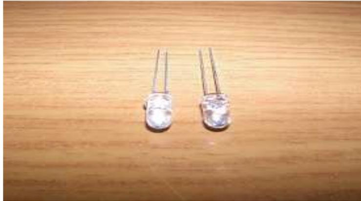
Fig. 4.15 Appearance of the infrared rays sensor
