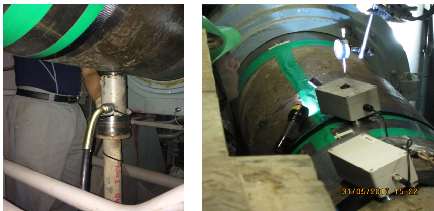
Fig. 4.1 Example: Hydraulic jacking up and dial gage for measurement
