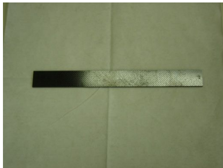
(a) NHT(Non-hole Tensile) specimen
