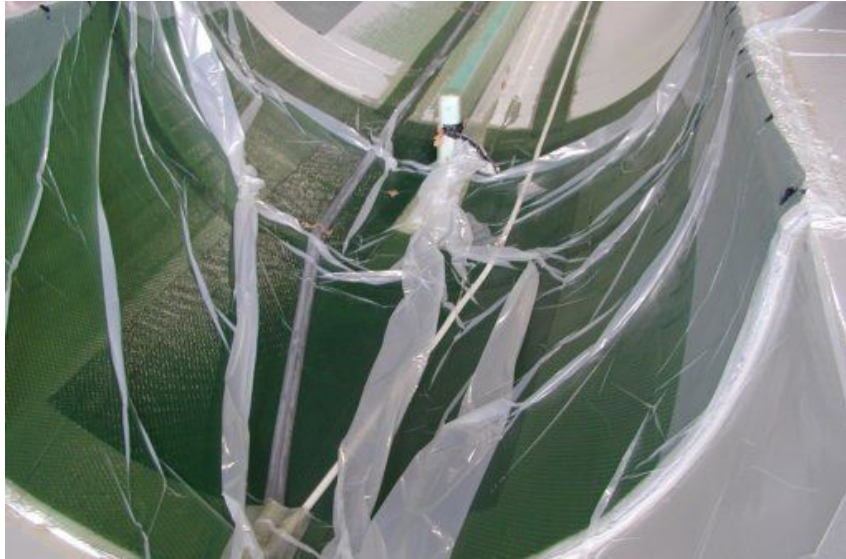
Fig. 25. Lay-up process of VaRTM process
