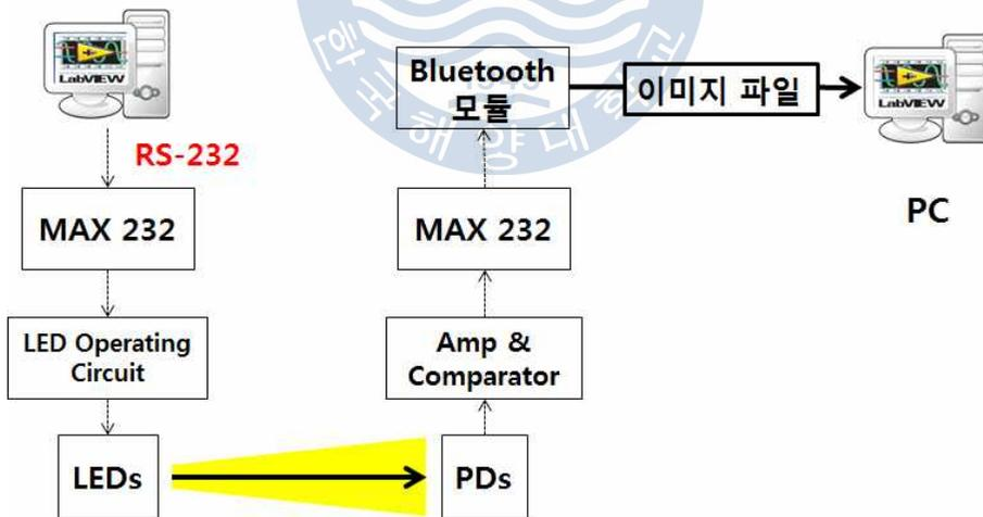
Fig. 16 System schematic for image transmission experiment
