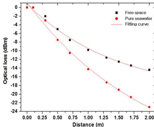
Fig. 23 Optical loss by distance at underwater
