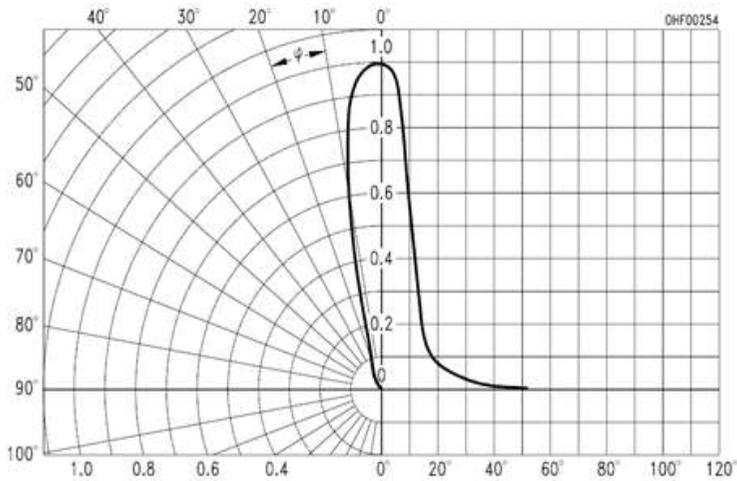
Fig. 11 Field angle of PD<sup>[25]</sup>
