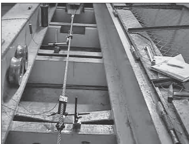
Figure 4 Acoustic method measurement set up. Display of the measurement part of the set up – microphones and deviation gauger.
