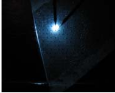
Fig.6.32 Emitting light of DH structure with In(0.5)Al(0.6)GaN active layer
