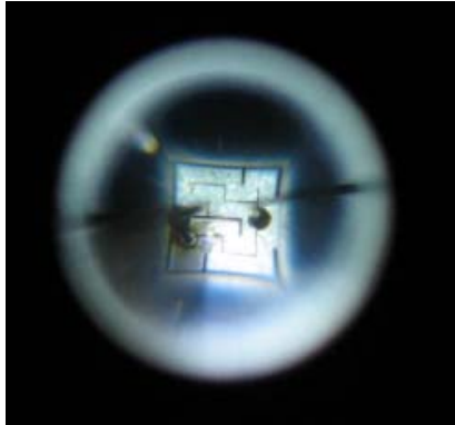
Fig.7.14 White emission of Phosphor-free LED Lamp
