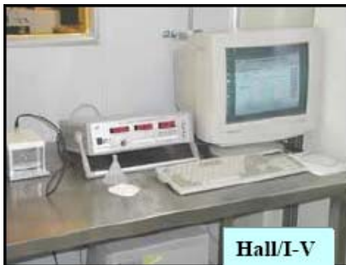
Fig.3.9 Hall Measurement System.
