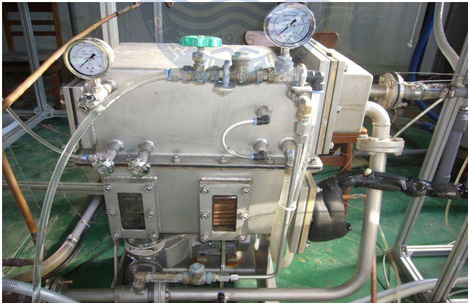
Fig. 3.18 Evaporator and Condenser
