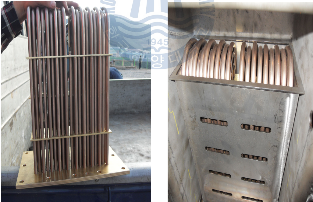
Fig. 3.5 Photographs of condenser unit
