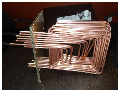
Fig. 3.3 Photographs of evaporator unit
