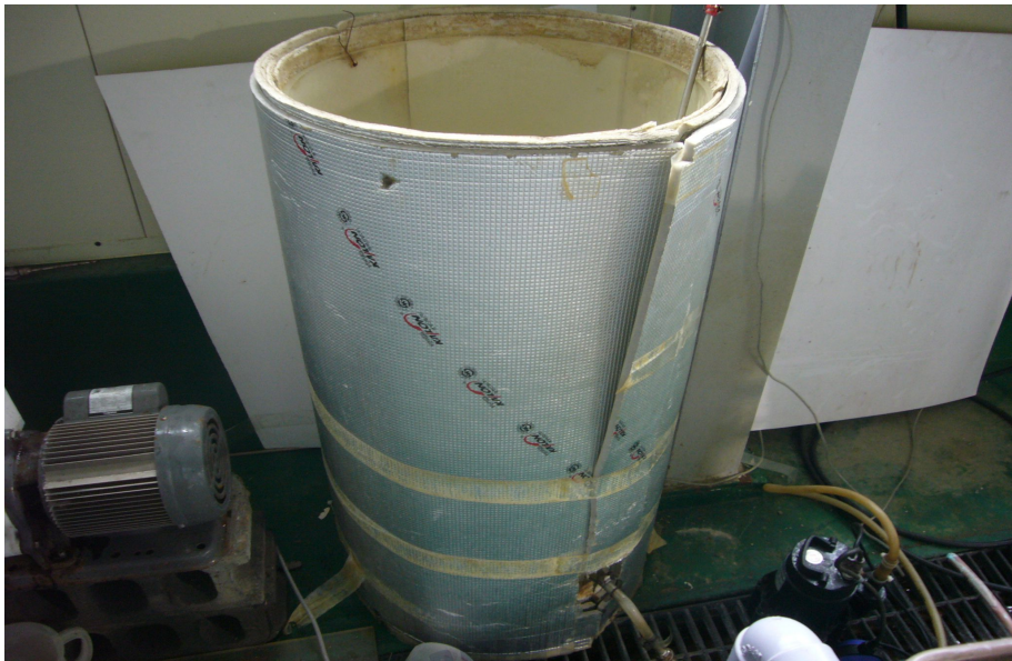
Fig. 3.23 Feed brine tank
