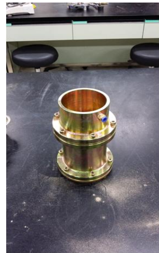
Fig. 4.22 Remolded process of constant head permeability test
