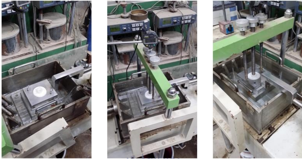
(a) Shear box installation (b) Saturation of sample (c) Completion
