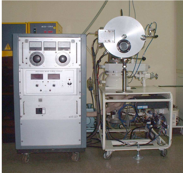
Fig. 3.1 Photograph of thermo-electron activated ion plating apparatus.
