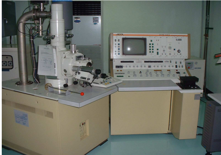
Fig. 3.3 Photograph of scanning electron microscope
