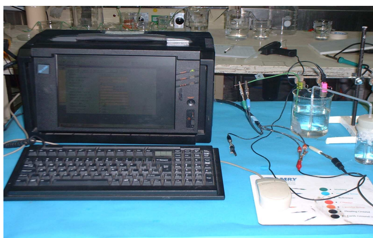
Fig. 3.7 Photograph of polarization test system
