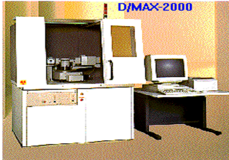
Fig. 3.5 Photograph of x-ray diffraction analysis apparatus
