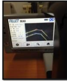
Weld bead inspection system
