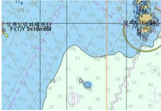
Fig. 4.12 Change of Isolated danger mark depending on shallow danger function (ECDIS Maker : MECys)
