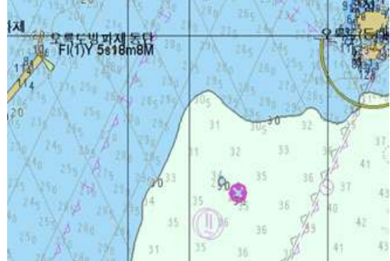
Fig. 4.12 Change of Isolated danger mark depending on shallow danger function (ECDIS Maker : MECys)
