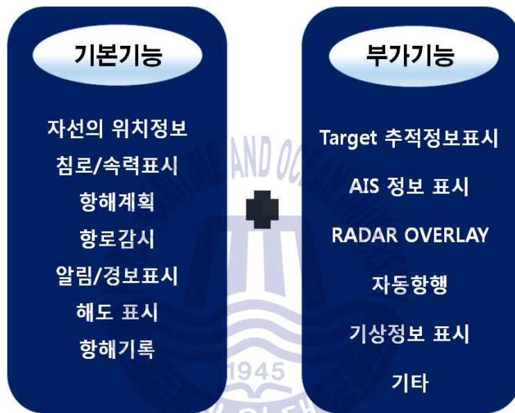
Fig. 2.2 Functions of ECDIS
