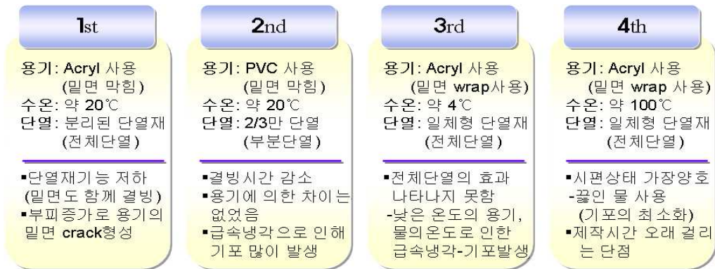
Fig. 3-8 Procedure of specimen preparation by trial and error
