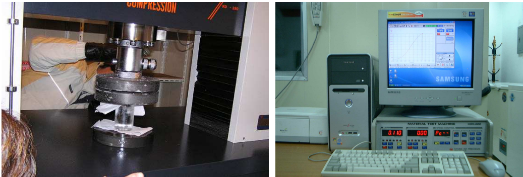
Fig. 3-2 The 20-ton class UTM for compression and bending tests
