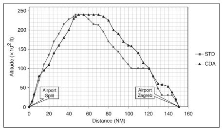
Figure 1 - Standard approach and continuous descent flight profiles
