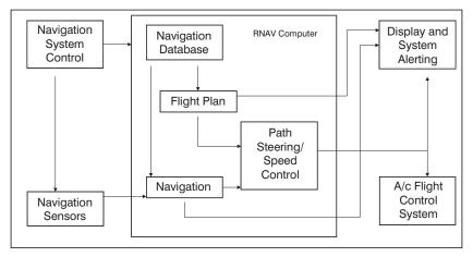
Figure 4 – RNAV system functions
