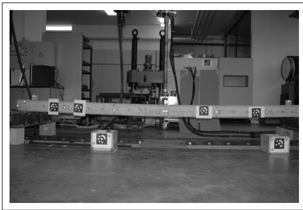
Figure 3 - Prefabricated pre-stressed concrete plate with measured marks
