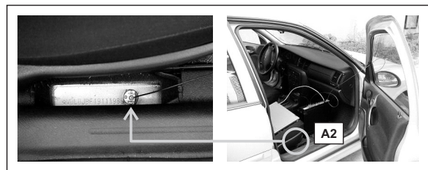
Figure 2 - Accelerometer A2 on the vehicle chassis
