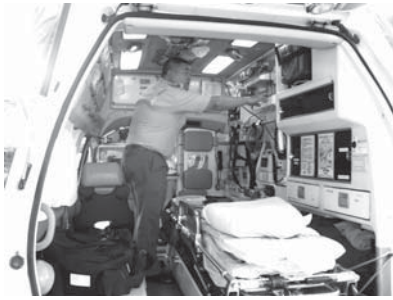
Figure 5. A standard Japanese ambulance, which has a small and narrow space around the patient.
