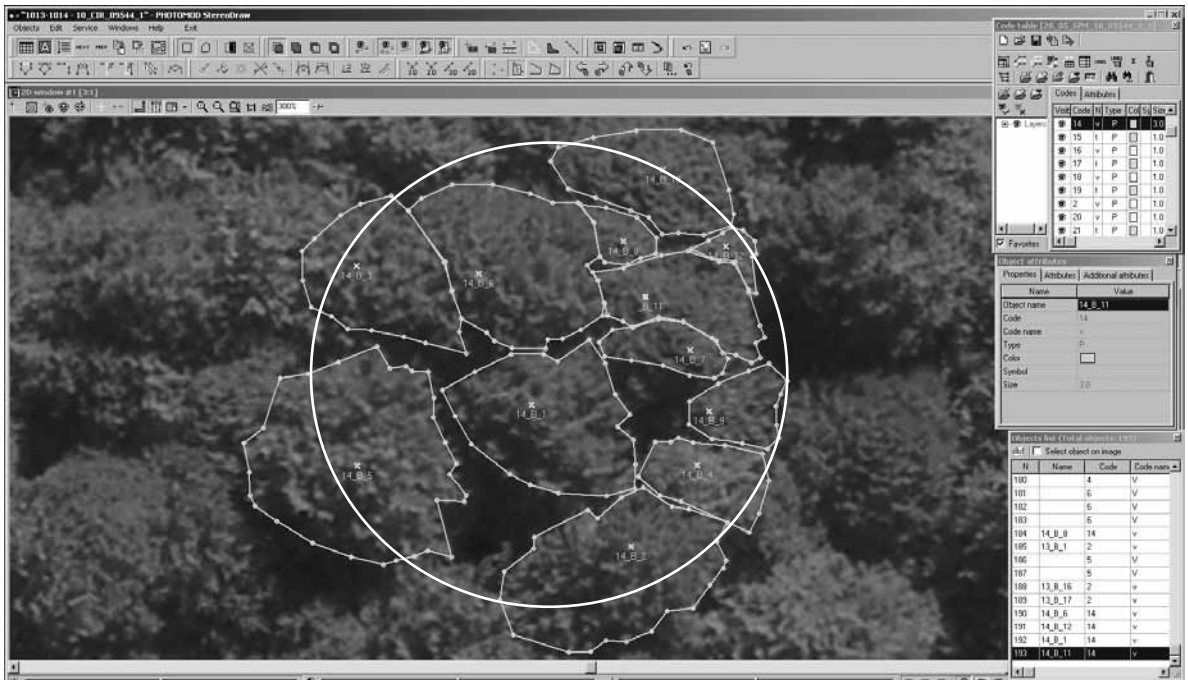
FIGURE 7 An example of a photogrammetric measurement of stand structure elements shown in model of CIR digital aerial images of GSD 10 cm in 2D window of StereoDraw module at magnification of 300 %.
