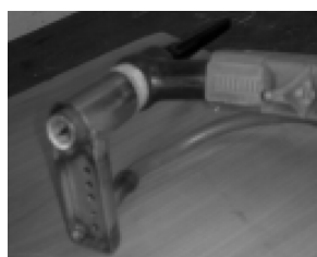
Slika 7. Naprava za sekundarnu zaštitu lica zavara Figure 7. Device for secondary protection of the weld face
