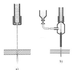
**Figure 1.** Scheme of the processing without abrasive water-jet a) and with abrasive water-jet b)
