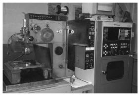
Figure 10. Spark erosion machine ANUC TAPE CUT-MODEL H
