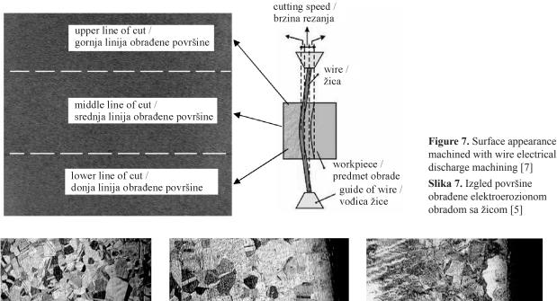
machined with wire electrical discharge machining [7] Slika 7. Izgled površine
