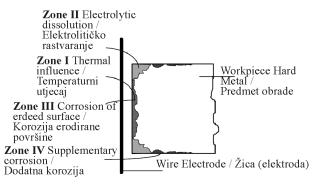
Figure 2. Characteristic zones on the hard metal machined surface [2]
