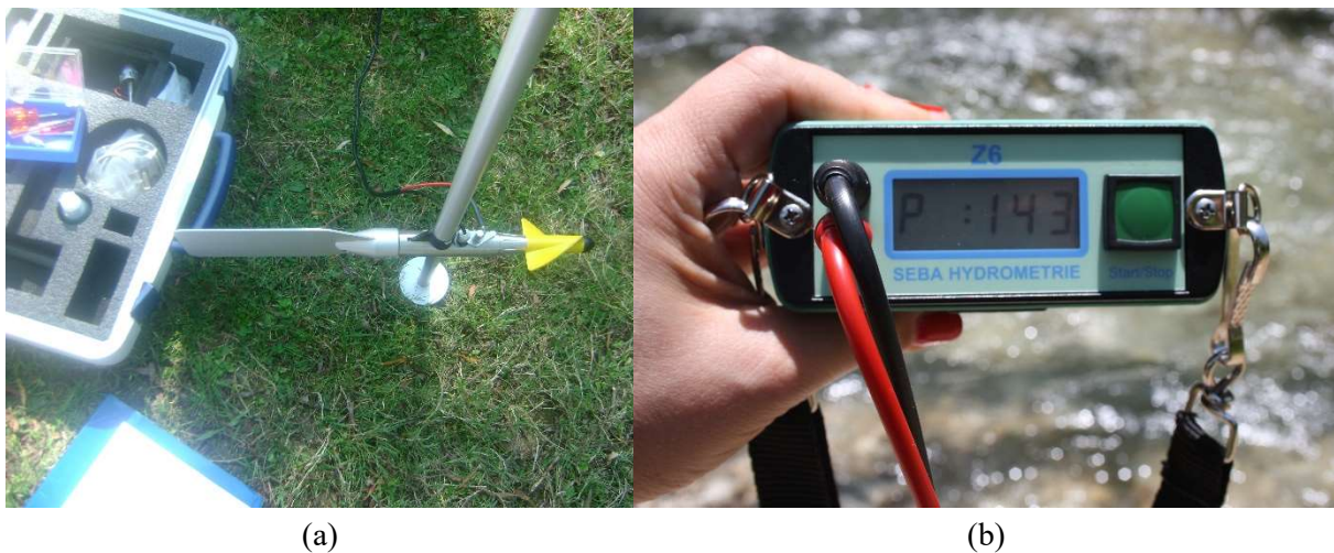
Figure 5.10 Universal Wing SEBA F1 (a) and counting device SEBA Z6 (b)
