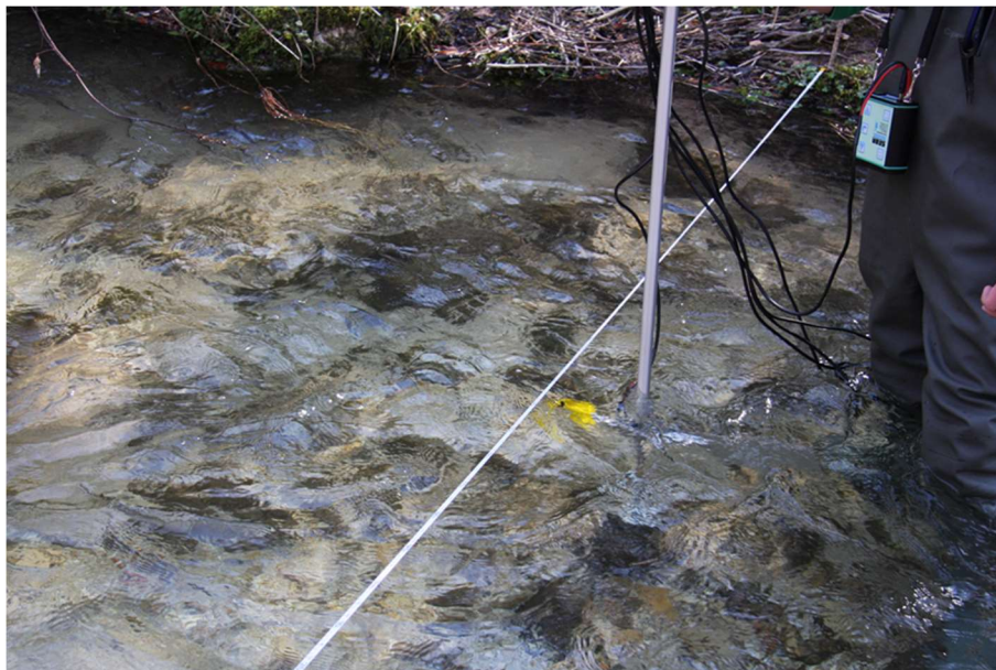
Figure 6.39 Current meter measurements by wading
