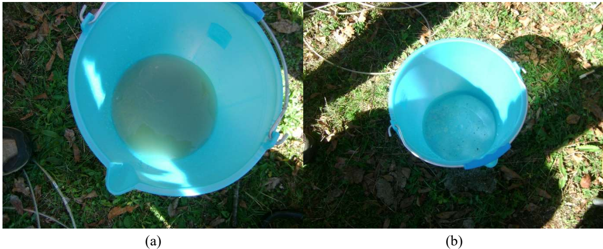
Figure 5.6 Well purging procedures for obtaining valid water samples from monitoring wells: before (a) and after (b) three well volumes removing (GW_02, May 2016)
