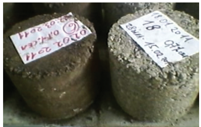
Figure 3. Stabilisation mix samples (slag on the left, and crushed stone on the right)
