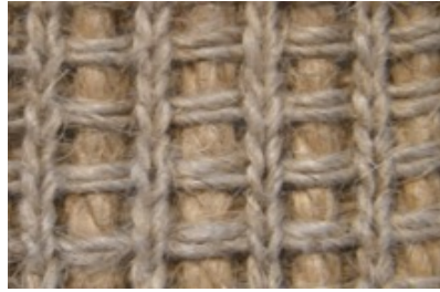
Figure 5: Sisal inlay/knitted flax 1x1 rib base structure
