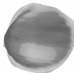
Figure 12. Grayscale 3D thermogram of the ballistic gelatin with resistor 7 active.
