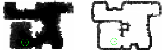
Fig. 4. Fuzzy occupancy grid-maps representing the empty (left) and occupied (right) space. Darker cells have higher degrees of certainty of being empty (left) or occupied (right). The green circle indicates the current robot position.
