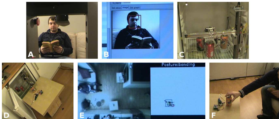
Fig. 10. Snapshots from the execution of the example run: (A, B) the PeopleBot and its on-board pan-tilt camera recognizing the person; (C) the fridge grasping the drink and (D) placing it on the docked PEIS-Table; (E) the stereo-camera for locating the position of the person in the home; and (F) the user receiving his drink.
