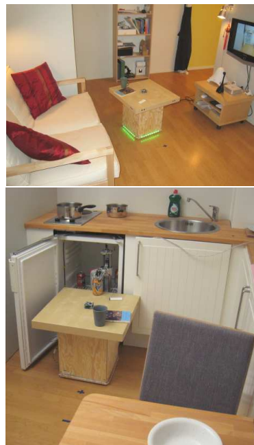
Fig. 8. Two views of the PEIS-Table operating in the PEIS-Home. Top: navigating inside the living room. Bottom: docked at the fridge.
